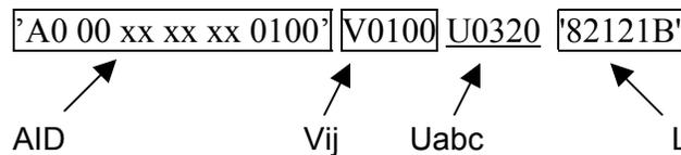
Note: Quotation marks (' and ') used above are not encoded within the LDS. They are shown to visually delineate hexadecimal characters.
