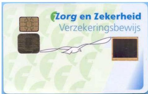
The Parkinson Pass contains both a built-in memory chip and a processor chip, the former linked to a sensor for biometric identification (fingerprint).
