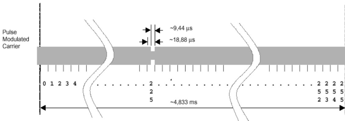
Figure 8 - 1 out of 256 coding mode
