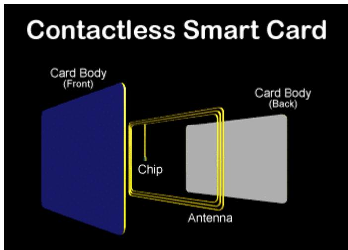
Figure 1 - Contactless card structure
