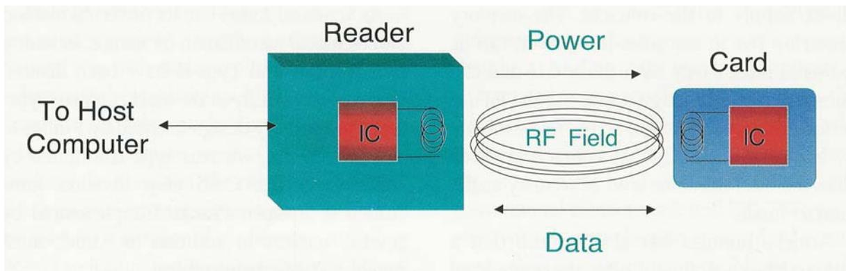
Figure 3 - Contactless card in a RF field
