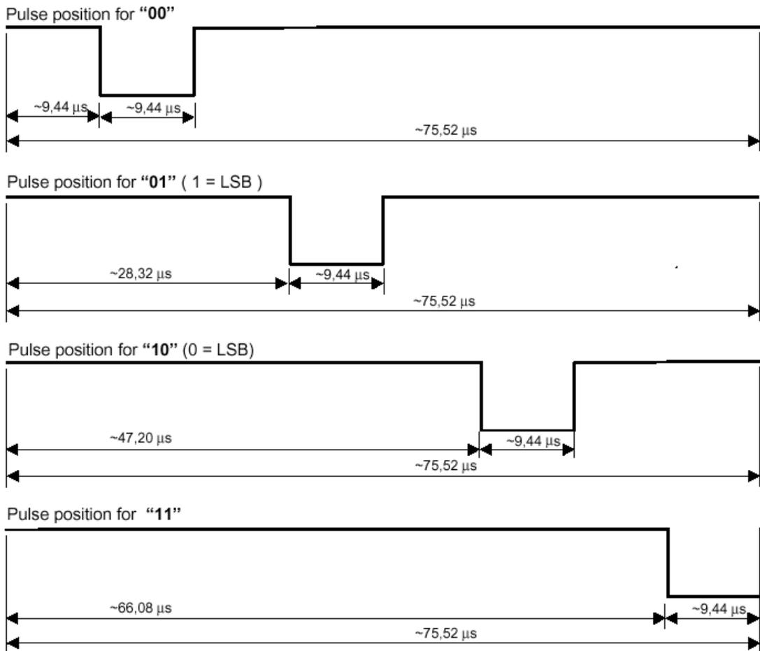
Figure 9 - 1 out of 4 coding mode
