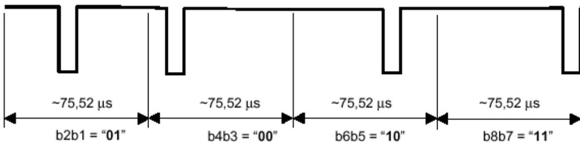
Figure 10 - 1 out of 4 coding example
