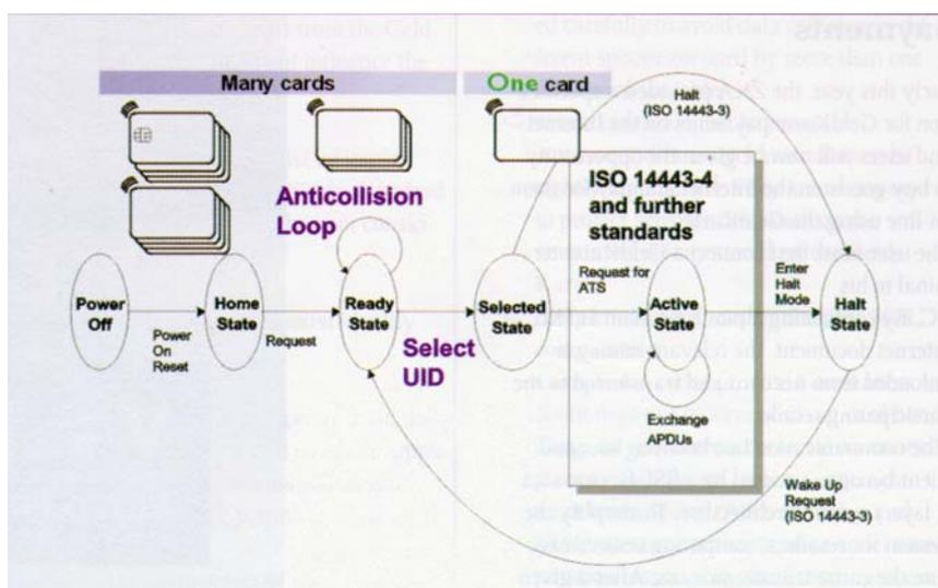
Figure 6 - State diagram for Type A cards
