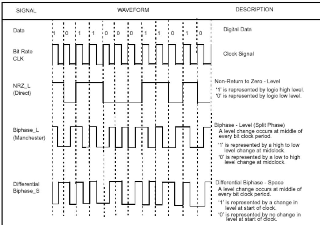
Figure 5 - Various data coding waveforms
