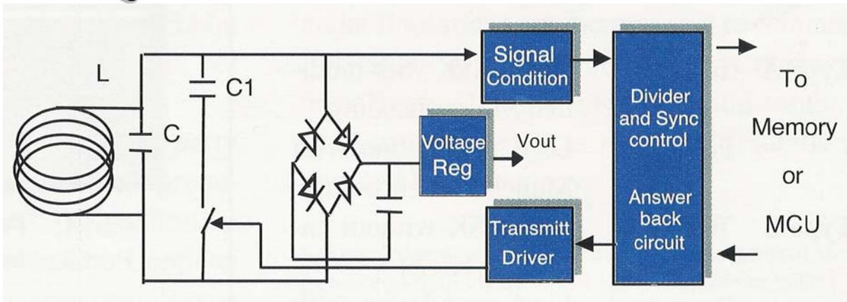
Figure 2 - Typical RF contactless receiver
