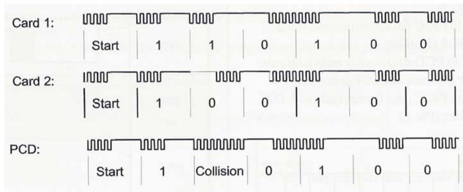
Figure 7 - Bit collision detection principle used by Type A cards
