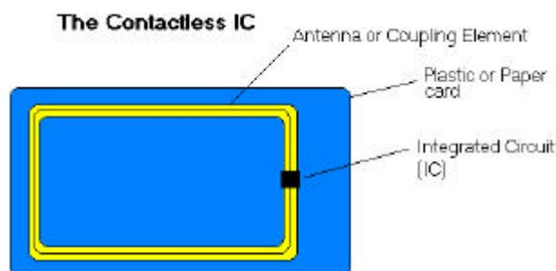
The main part of the contactless IC is a low-power IC that controls the communication with the machine (RF) reader. The IC also contains memory of some type to hold data. There are three types
